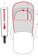
Push drink bladder into the slot on the carry system interior and secure with the strap and flat-front buckle.
