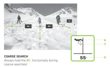
From a distance of approx. 55 m from the victim, the direction arrow (7), relative position (6), and distance indicator (9) appear on the screen and lead you along the field line to the target location.
